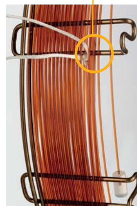
String indicates where the analytical column begins.
