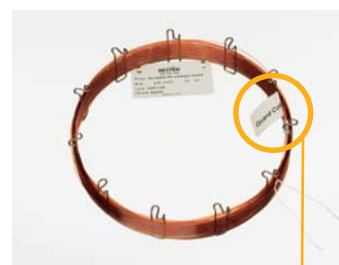
Tag indicates guard column end.
